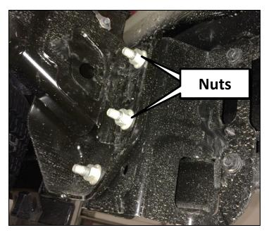
Install the bumper step onto the studs. Then reinstall the factory nuts that were removed in step one. Fully tighten the hardware.
